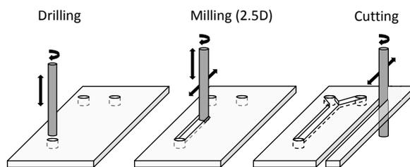
Figure 4. Versatile glass machining by SACE: drilling, milling and cutting by the same technology on the same setup.
