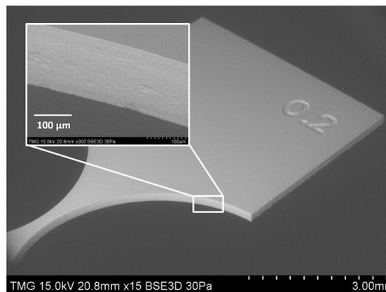
Figure 5. Smooth cutting of glass ( $R_z < 1 \mu\text{m}$ ) by SACE technology.
