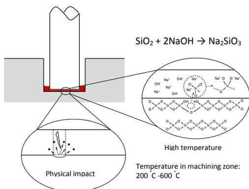
Figure 2. Electrochemical discharge machining mechanism of SACE technology on a glass substrate.
