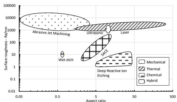
**Figure 1.** Surface roughness Ra/nm vs. aspect ratio for different glass drilling methods, categorized in four categories (Mechanical, Thermal, Chemical and Hybrid).
