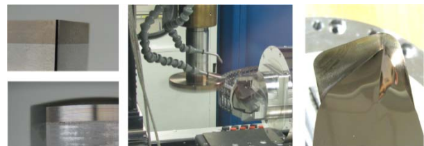
Figure 4. Steel moulds with high-build eNiP-layer, up-fly cut setup and up-machined structured free form
