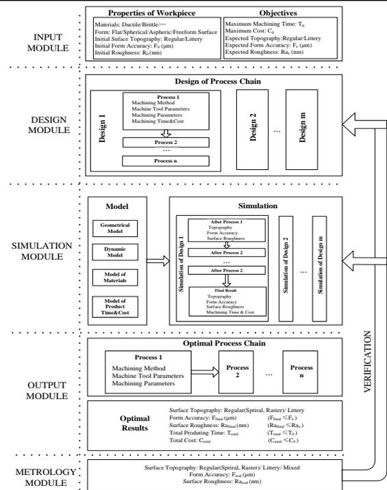
Figure 1. A framework of process chain optimization system.
