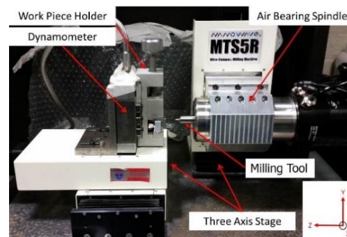
Figure 1. Nanowave MTS5R Micro-milling system with \Phi 0.5 mm single crystal diamond tool and air bearing spindle.
