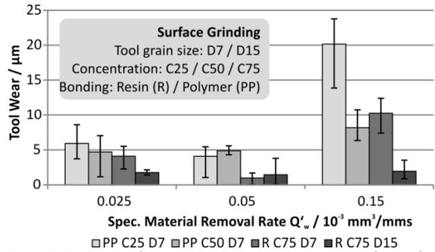
**Figure 3.** Tool wear of resin and polymer bonding systems after surface grinding of CVD-SiC.
