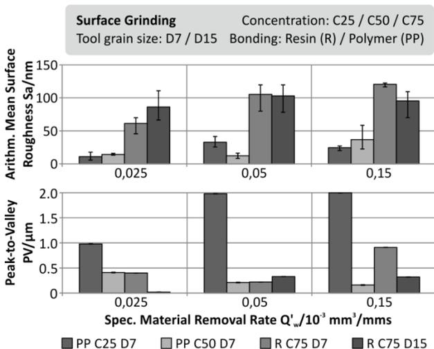
**Figure 2.** Surface roughness ( $S_a$ ) and shape accuracy (PV) of ground plano surfaces in CVD-SiC using soft bonding systems.
