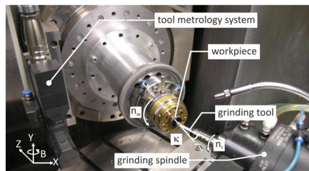
Figure 1. Experimental grinding set-up with in-situ tool metrology.
