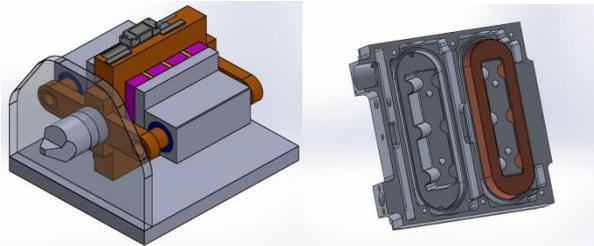
Figure 3. Schematic design of FTS with air bearings and a linear motor composed by two coils and permanent magnets.
