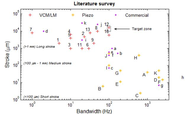
Figure 2. Characteristics (bandwidth and stroke) of analysed solution for Fast Tool Servo, the references are listed in next table.
