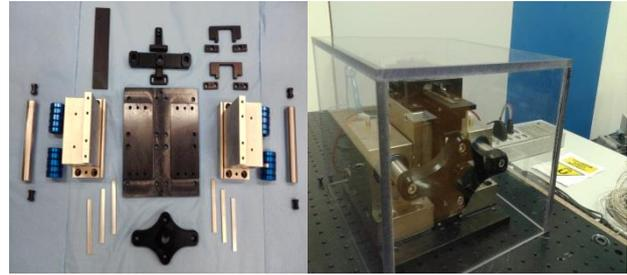
Figure 5. Prototype of FTS for large displacement, parts and assembly.
