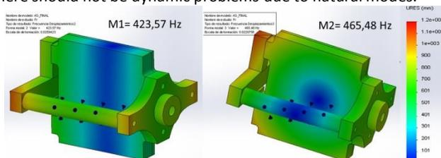
Figure 4. First two natural modes of vibration of designed structure.
