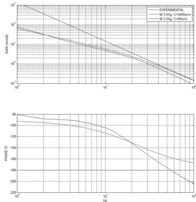
Figure 6. Experimental response of system in open-loop.
