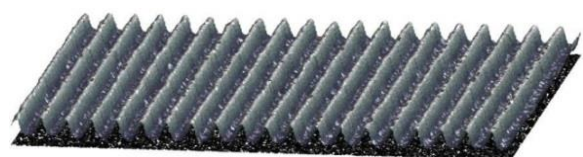
Figure 1. Model of a 2\ \mu\text{m} \times 4\ \mu\text{m} sinusoidal grating with a 180 nm height.
