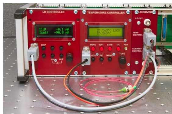
Figure 1. Laser diode control electronics: left to right are the current source with current controller, the temperature controller and the diode housing.
