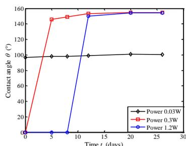
Figure 2. Time dependent contact angle of ablated surfaces.
