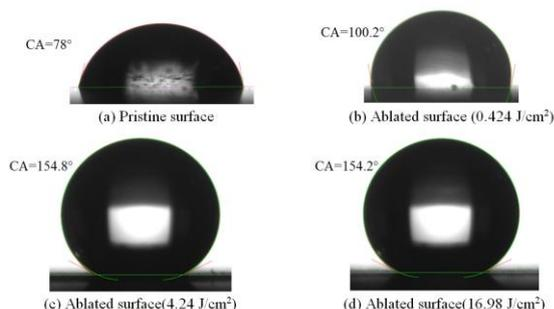
Figure 1. Contact angle of the ablated stainless steel.
