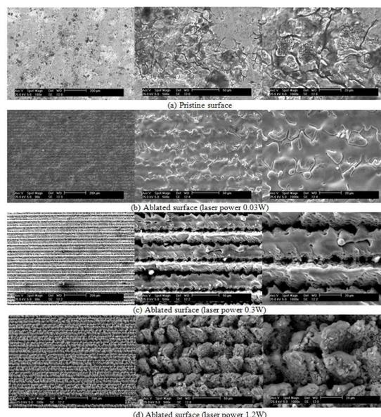
Figure 3. SEM images of the machined stainless steel.
