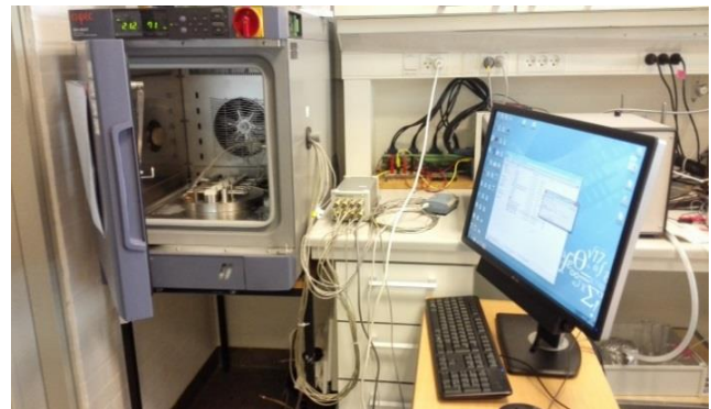
Figure 1. Set-up for length measurements in the climatic chamber.
