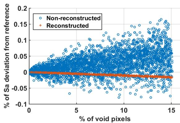
Figure 2. Distribution of Sa parameter with Random-based algorithm on turned surface with a reference Sa of 1.354 μm.
