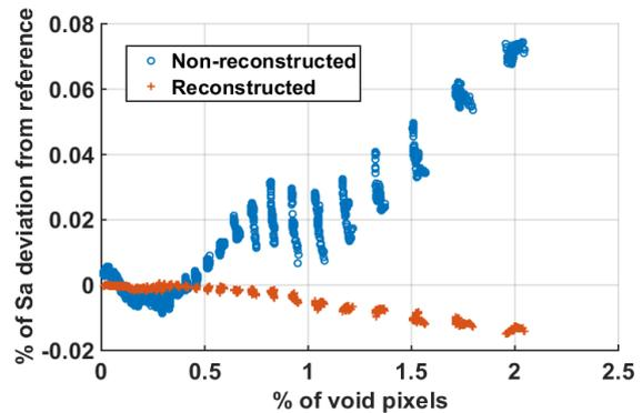
Figure 3. Distribution of Sa parameter with slope-based algorithm on a turned surface with a reference Sa of 1.354 μm.
