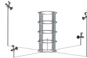
**Figure 2.** An example setup showing four sensor heads measure glass targets mounted onto the structure being measured.
