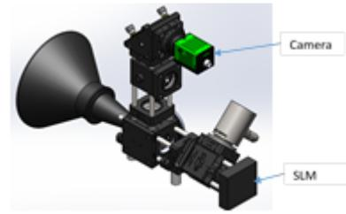
**Figure 1.** Prototype sensor head developed at NPL for multi-beam FSI measurements. A camera system is employed to detect where in the SLM FoV the targets are located. Both the camera and SLM share a similar optical axis to ensure easy transformation between the two 2D coordinate systems.
