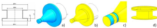
Figure 2. Machining of a gold “thin wall” part, a) Turning of brass mandrel, b) Gold plating, c) gold machining, d) selective dissolution of brass mandrel.
