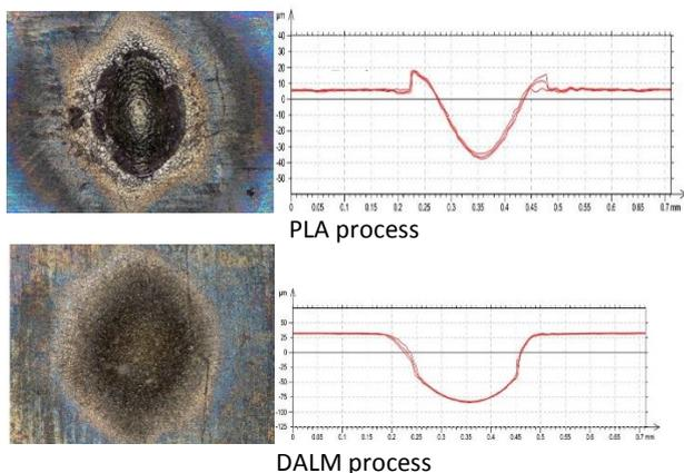
**Figure 3.** Images taken by the infinite focus optical microscope (Number of laser and droplet pulse = 125; Laser frequency = 10Hz; Droplet frequency = 10Hz; Laser fluence = 5J/cm<sup>2</sup>).
