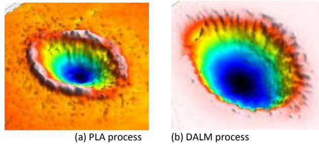
**Figure 4.** 3d profile of the hole machined with PLA and DALM.
