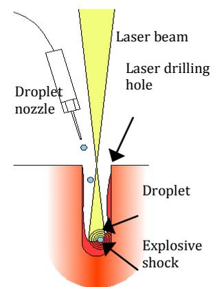
Figure 1. Schematic of DALM setup
