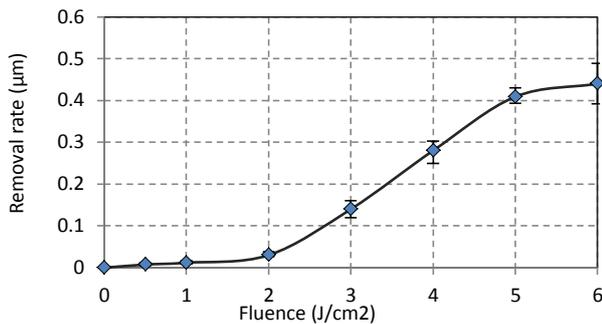
**Figure 2.** Graph showing effect of laser fluence on removal rate for DALM (No of laser and droplet pulse = 250; Laser frequency = 10Hz; Droplet frequency = 10Hz).
