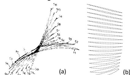
Figure 1(a) Top view of the stacked airfoil segments for a blade[7].
