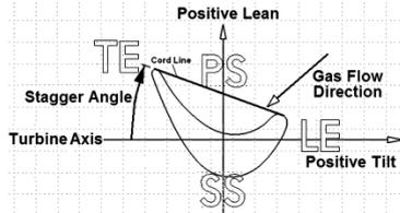
Figure 2. The geometrics of the airfoil segment[6].
