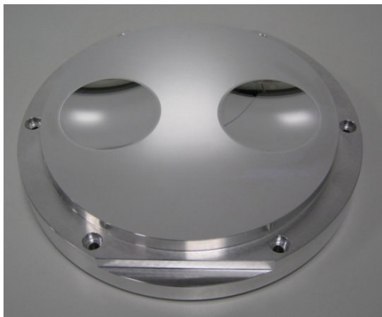
Figure 3. Off-axis-sphere for demonstrating the freeform capabilities of the UPC 400.
