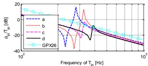
Figure 6. Frequency response from inner rotor torque  $T_{in}$  to inner rotor position  $\theta_{in}$  for magnetic gears a-d and the GPX 26 mechanical gear.
