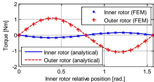
Figure 3. Magnetic gear torque as a function of the inner rotor position relative to the outer rotor.
