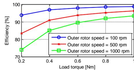
Figure 5. Efficiency of magnetic gear (a) in Table 2.
