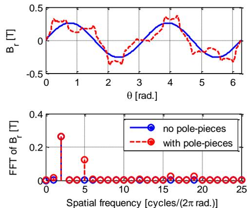
Figure 2. Airgap radial magnetic flux density  $B_r$  and its harmonic content, produced by the inner PM array of the gear in Fig. 1 (b).
