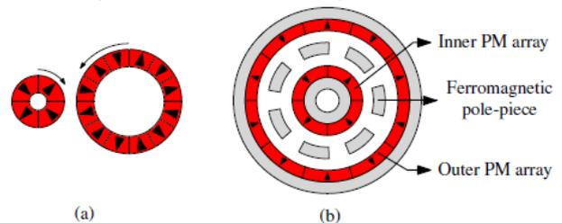
Figure 1. Magnetic gear: (a) spur-gear based topology. (b) Investigated topology.
