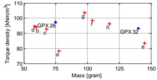
Figure 4. Torque density and mass of the gears in Table 2.
