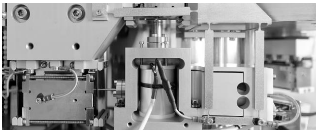
Figure 3. Existing 2DOF Sensor-Actuator Unit with patented tilt to horizontal decoupling.
