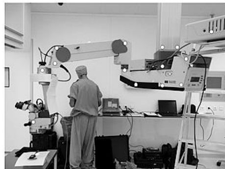
Figure 2. Modal measurements of the microscope. Dots indicate sensor points.
