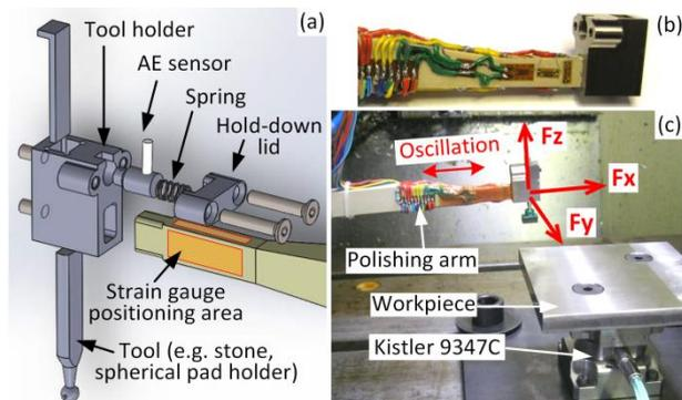
Figure 2. CAD model of the polishing arm with integrated sensors (a), manufactured arm (b), setup of dynamic performance verification (c).
