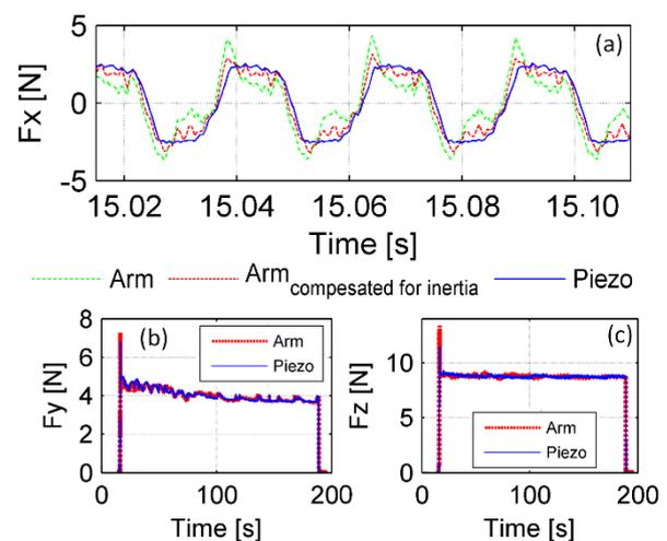
Figure 3. The effect of inertia on  $F_x$  force measurements during arm oscillation  $3000 \text{ min}^{-1}$  (a), comparison of forces measured by the arm and reference piezoelectric dynamometer during RAP of a rotating workpiece:  $F_y$  (b) and  $F_z$  (c).
