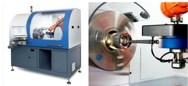
Figure 1. STRECON's Robot Assisted Polishing (RAP) machine tool (left), working space with polishing module utilizing oscillating tool (right).
