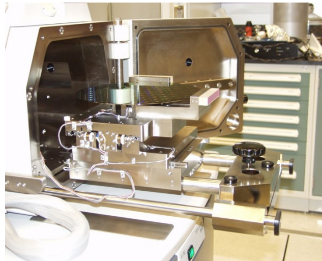
Figure 1. The sample stage with a 300 mm wafer and the high-precision sample exchange mechanism.
