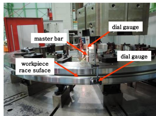
Figure 1. Previous experimental setup for the error subtraction method
