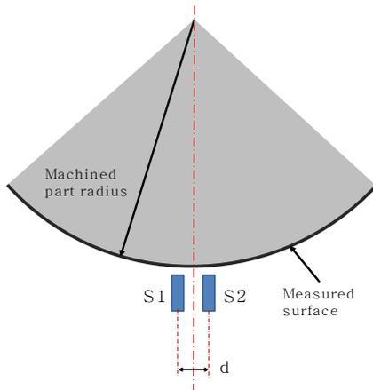
**Figure 3.** The measurement setup schematic for proposed two-probe differential method
