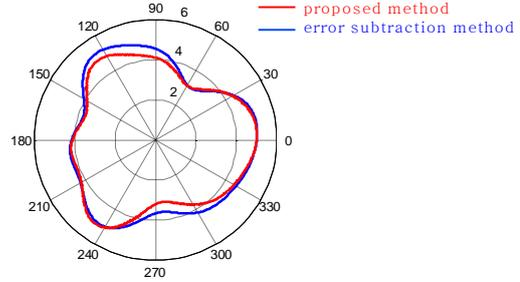
(b) Rotary table radial error motion measurement results
