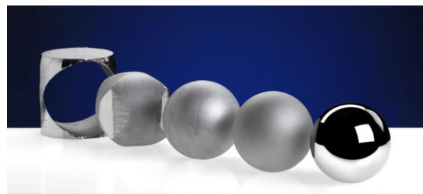
Figure 1. Hollowed ingot, cut, turned, lapped and polished sphere
