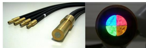
Figure 1. On the left picture, the fiber optic bundle with one common input structured in four quadrants and four outputs. The ferrule serves as a holder. On the right picture, the light of four power LEDs of different colours is injected from the outputs solely to distinguish the quadrants geometry on the input.
