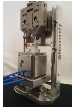
Figure 4. The test instrument equipped with the 3-axis force sensor
