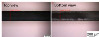
**Figure 3.** Optical images of the cutting kerf showing the clean surface without cracks and chippings.
