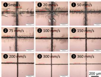
**Figure 2.** Optical images of a cross ablated with focus at glass top surface using a single scan under varied scanning speeds.
