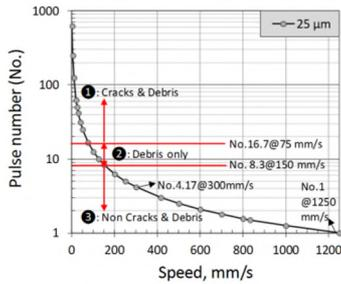
**Figure 1.** Plot of pulse number versus scanning speed showing no cracks and debris produced under high laser scanning speed.
