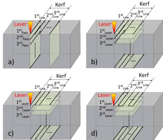
**Figure 4.** Schematic illustration for each scanning mode. a) *Group mode*: Scanning of first line with multi-passes, then scanning next line with the same multi-passes in the same direction. b) *Merge mode*: Scanning of multi-lines with one pass, then scanning multi-lines again with next pass layer by layer in the same direction. c) and d) *Raster mode*: Similar multi-lines scanning to merge mode but able to scan in two direction or continuous scanning.
