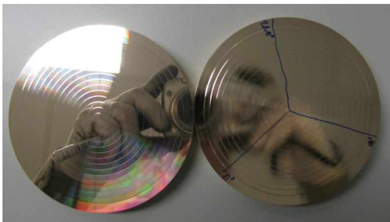
Figure 3: Hardened metal alloy machined with standard diamond tool (right) and with macle diamond tool (left).
