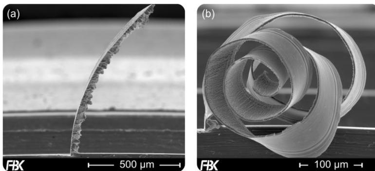
Figure 3: (a) QST with an undeformed chip thickness  $h = 10 \mu\text{m}$  and (b) an undeformed chip thickness  $h = 1 \mu\text{m}$ .
