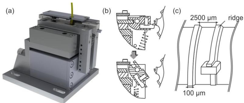
Figure 2: (a) Perspective view of the assembly (b) Details of the release mechanism (c) Process conditions in orthogonal cutting.
