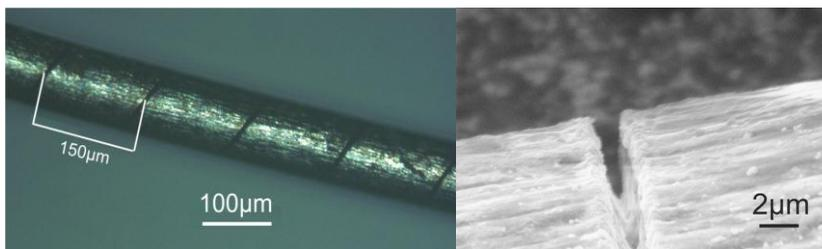
Figure 3: Photomicrograph of the laser structured fiber (left), SEM image showing the structured gap in detail (right)
