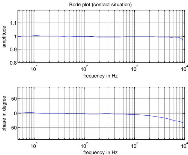
Figure 3: Bode plot in contact situation
