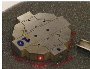
Figure 2: Sample structure designed to eliminate the assembling and mounting influences out of the modal measurements
