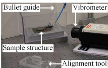
Figure 3: Innovative modal experiment launching bullets to excite the structure in the desired frequency range
