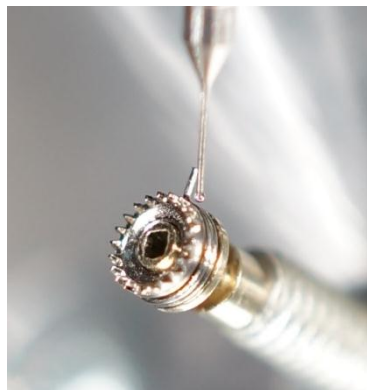
Figure 4: gear wheel with a side index shaft and square center hole measured with our \mu\text{CMM} fitted with a \varnothing = 0.2 \text{ mm} probe
