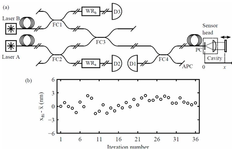
Figure 2: (a) Dual laser optical setup capable of measuring absolute distances with nanometer repeatability. Both lasers are wavelength stabilized to two reference gas cells  $WR$ . (b) Repeated measurement of the absolute position showing an uncertainty of  $\pm 3$  nm.
