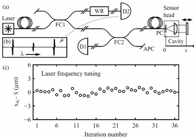
Figure 1: (a) Single laser fiber-optic setup for the measurement of incremental displacements of a target mirror. The laser light is routed through fiber couplers FC and detected at the detectors D. Fiber end and mirror form a low-finesse Fabry-Pérot cavity. (b) Gas cell demodulation signal as a function of the wavelength  $\lambda$ . (c) By tuning the laser wavelength, the absolute position  $x_{\text{fit}}$  can be measured with an uncertainty of about  $\pm 1 \mu\text{m}$ .
