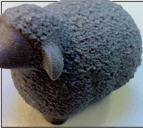
Figure 2: FDM part demonstrating how layer-structure can be camouflaged by surface structuring.
