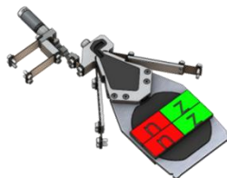
Figure 4: A detailed view of the drive train of one of the the pump valves
