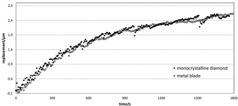
Figure 3: Repeatability of trigger position relative to first trigger position. The major influence harming performance is the duration of every single measurement since heating of the light barrier cause significant errors. A typical measuring cycle takes less than 2 minutes thus the visible and detected dislocation of the trigger position is of minor relevance.
