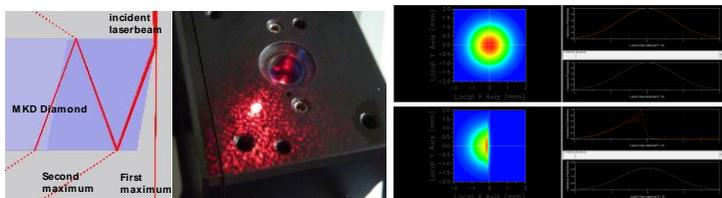
Figure 2: Reflection of the beam (left), real refraction (middle) and simulated intensity at the sensor (right).
