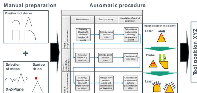
Figure 4: Measuring procedure.
