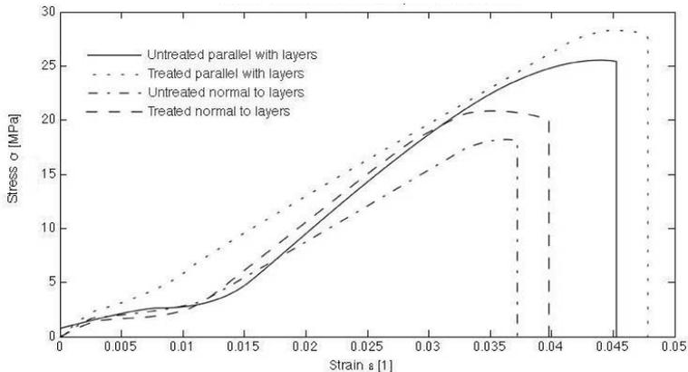
Figure 2: Normalized & averaged stress-strain, virgin and vapour treated specimens
