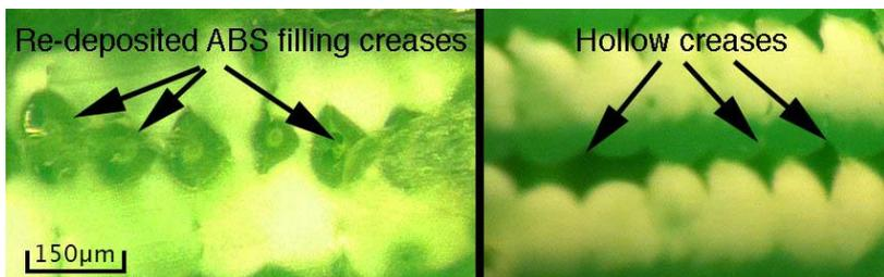
Figure 3: Cross-sectional dissection Left: vapour treated Right: untreated
