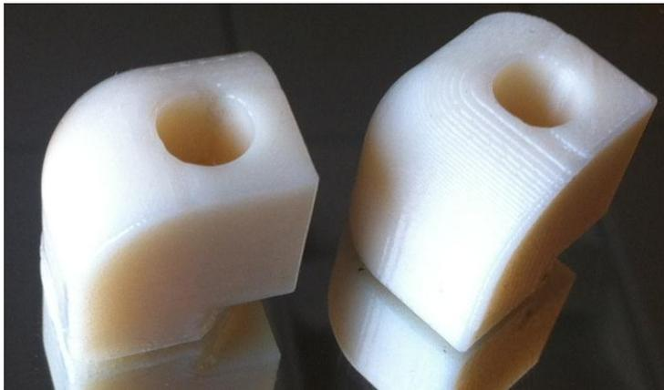
Figure 1: Left: Geometry #1, vapour treated Right: Geometry #1, untreated
