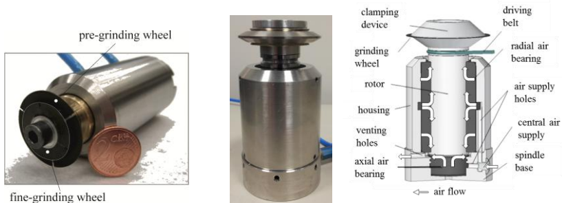
Figure 1: grinding spindle with 12 mm rotor and two grinding wheels (left), prototype of the new developed air bearing spindle (middle) and model (right) (one grinding wheel)
