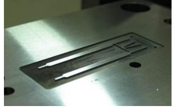
Figure 3: Mould insert milled in tool steel for the replication of the reference structure by injection moulding
