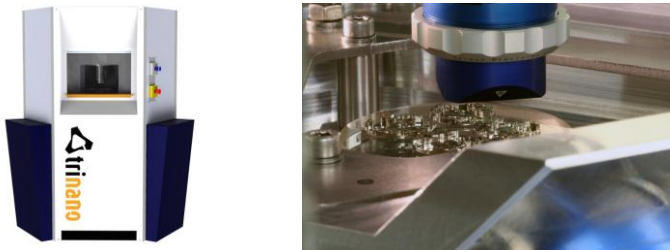
Figure 1. Left side: TriNano CMM (artist impression), Right side: measurement using the Gannan XM probe.
