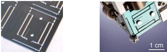
Figure 1: Photos of a flexure slab of the sugar cube Delta-Robot (left) and the sugar cube size Delta-Robot (right) [3]
