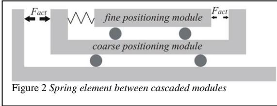
This paper investigates the possibility to make use of the actuators of the coarse positioning module to accelerate the fine positioning
