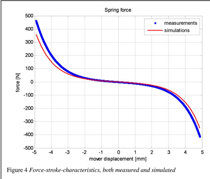
stiffness) reaches its minimum value. This configuration effectively reduces the disturbance forces transmitted by the coarse positioning module around the neutral position.
