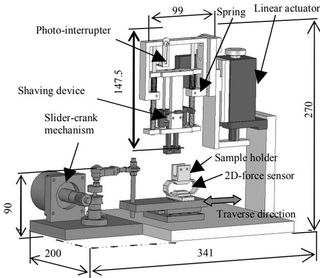
Figure 1: Structure of rock surface shaver
