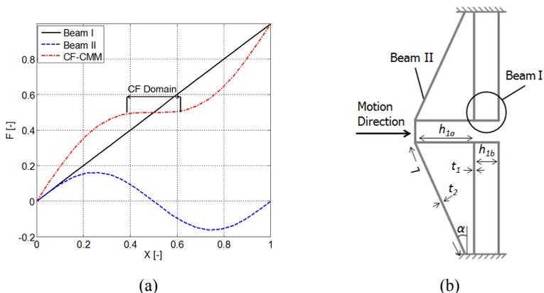
Figure 1: (a) Predicted force-deflection behaviour and (b) concept of the constant force carbon-nanotube-based compliant micro mechanism (CF-CMM).
