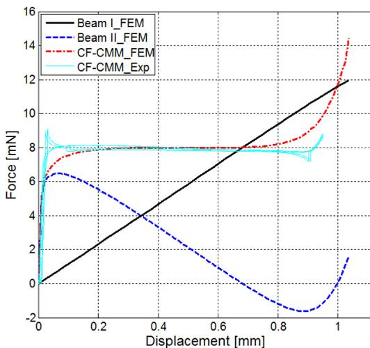
Figure 3: Force-deflection of the carbon-nanotube-based CF-CMM from the measurements and finite element modelling.
