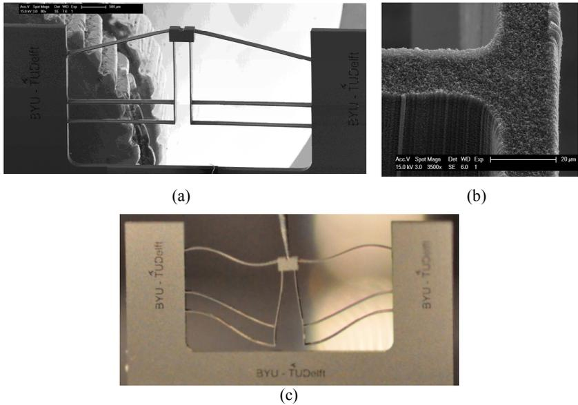
Figure 2: (a) Front view and (b) close-up of CF-CMM fabricated in the CNT-M process and (c) the deflection during the measurement.
