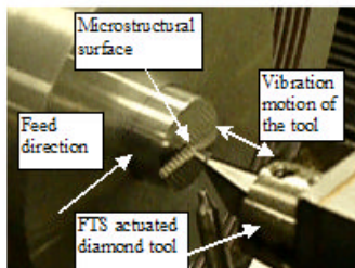
Figure 1: Graphical illustration of fast tool servo machining of microlens array
