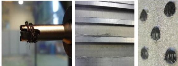
Figure 1: Typical problems of FRP material machining by cutting.
