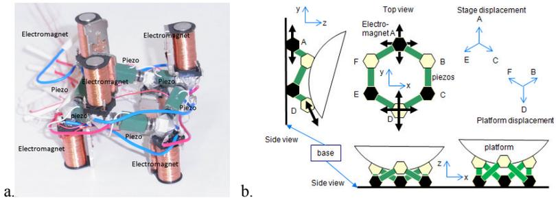
Figure 1: (a) Photo of the 6-DOF stage and (b) schematic diagram of the stage
