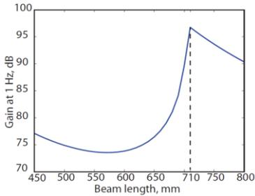
Figure 7: Optimal gains for different beam lengths with PID control.
