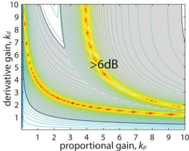
Figure 5: Constraint 2: Closed-loop frequency response < 6 dB..
