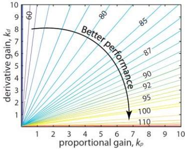
Figure 3: Objective: Open-loop gain at 1 Hz [dB].
