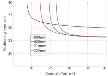
Figure 8: Pareto curves for different beam lengths with H<sub>2</sub> control.
