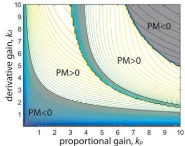
Figure 4: Constraint 1: Positive phase margin (PM>0).
