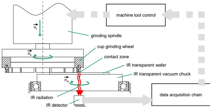
Figure 1: Schematic diagram of the temperature measurement and control system
