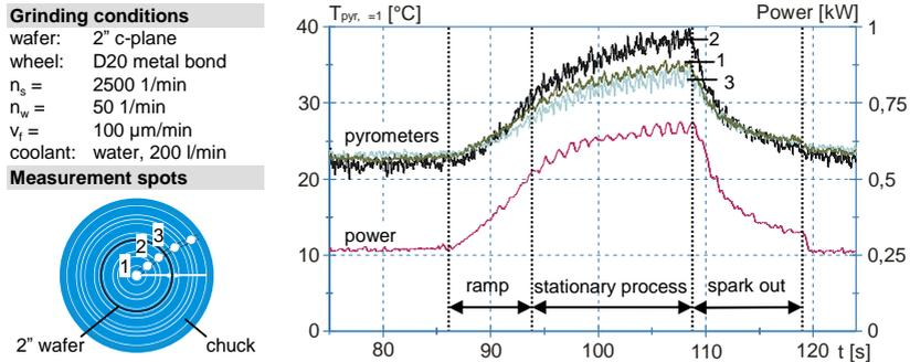
Figure 3: First grinding tests – sample measurement
