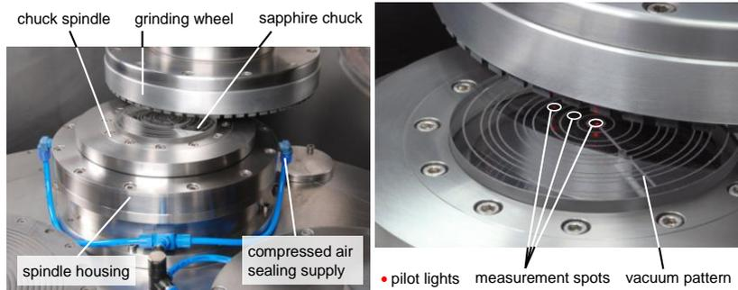
Figure 2: Realised wafer chuck system
