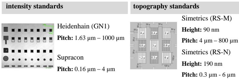
Figure 5: pitch standards for the measurement series and representative pictures
