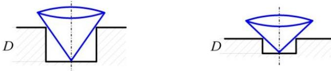
Figure 4: Examples of influences on optical structure resolution
