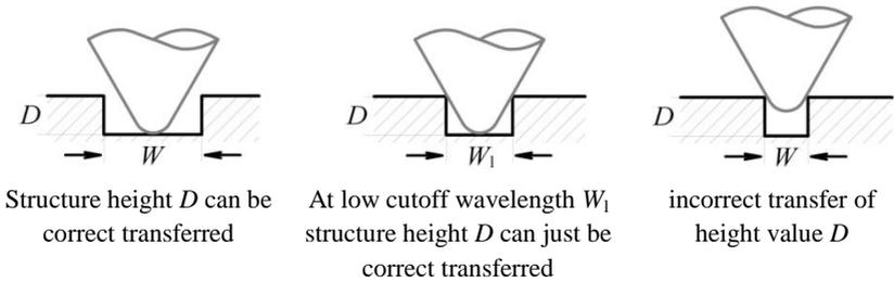
Figure 1: Description of the cutoff wavelength for tactile probing [ISO 25178-601]
