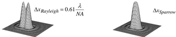
Figure 2: Comparison of the two resolution definitions
