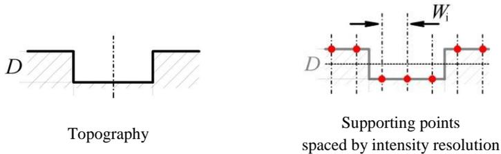
Figure 3: Relationship between intensity resolution and topographic resolution
