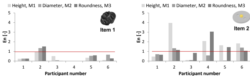
Figure 3: The quality of the measurements from the participants can be judged by calculating the E_n . Hence it is done for the two items and their measurands for six participants through the intercomparison. No data was acquired from participant number 4 for item 1.
